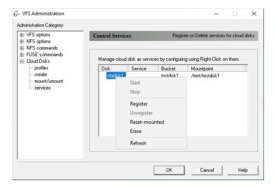
4. Try to Start service after Reset-mounted completed successfully.
